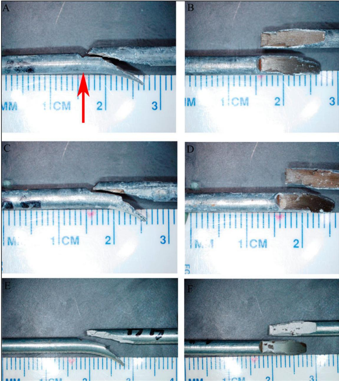
**Figure 7: Micrograph of Regular 0.136" diameter, 225ksi UTS Core Wire After Charpy Impact Testing. (A) and (B): 8°F, (C) and (D): 32°F, (E) and (F): 70°F. Arrow in (A) Indicates Notch Position.**
