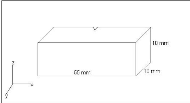
**Figure 1: ASTM standard V-notch Charpy test specimen**
