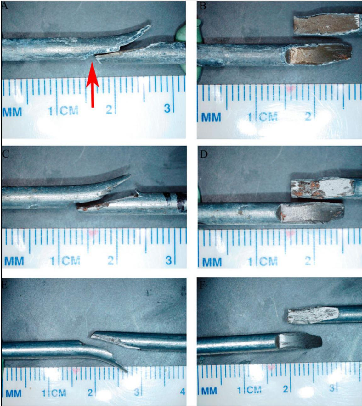
**Figure 4: Micrograph of Special 0.1493" Diameter, 275ksi UTS Core Wire After Charpy Impact Testing. (A) and (B): 8°F, (C) and (D): 32°F, (E) and (F): 70°F. Arrow in (A) Indicates Notch Position.**
