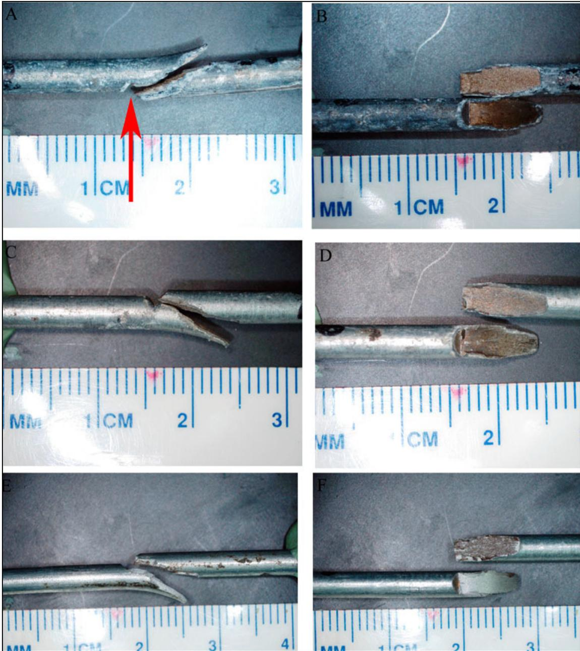
**Figure 5: Micrograph of Regular 0.1493" diameter, 220ksi UTS Core Wire After Charpy Impact Testing. (A) and (B): 8°F, (C) and (D): 32°F, (E) and (F): 70°F. Arrow in (A) Indicates Notch Position.**
