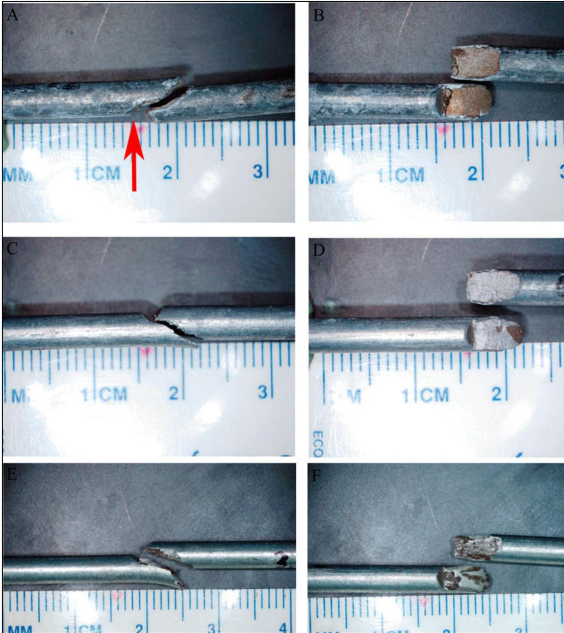
**Figure 6: Micrograph of Special 0.136" diameter, 285ksi UTS Core Wire After Charpy Impact Testing. (A) and (B): 8°F, (C) and (D): 32°F, (E) and (F): 70°F. Arrow in (A) Indicates Notch Position.**
