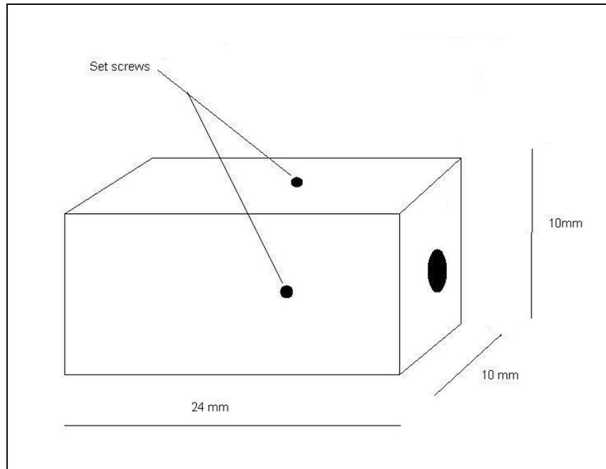
**Figure 2: Specimen holder for Charpy impact testing of wire samples**
