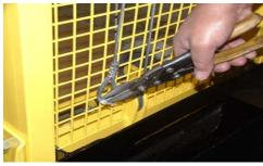
**Step 7.** Cut plastic tie holding lifting cable.
