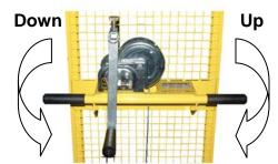
Turn winch crank clockwise to elevate the load, while watching for overhead obstructions. Turn winch handle counter clockwise to lower the load.
