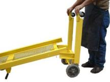
**Step 3.** Next, insert base into the mast as shown. Secure the tray to prevent it from sliding down during this operation.
