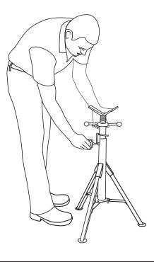
5. To lower jack head, lift both I.D. barrel and lock washer to loosen barrel. While holding lock washer lower I.D. barrel to desired height. Release lock washer to secure I.D. barrel.
