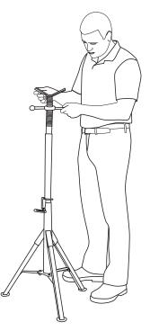
To position jack to desired height, loosen set screw and lift I.D. barrel. Lock washer will unlock when I.D. barrel is being raised and will grip automatically with the slightest load pressure.
