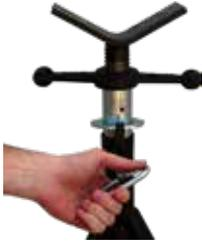
Tighten set screw so that the head cannot come out of stand.
