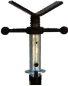
Vee head assembly can be locked in the jack for transportation. Position locator hole in ID tube so that it is in-line with set screw.
