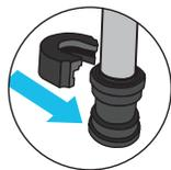
**TO REMOVE THE SIMPush™ FITTING, SIMPLY SLIDE THE REMOVAL TOOL ONTO THE COLLAR AND PULL**
