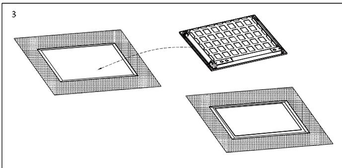
3. Place the panel into the flange kit and connect the input lines. Installation complete. (Fig 3)
