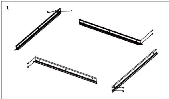
1. Remove accessories from the package carefully. Put together the four-piece drywall flange kit by using the supplied Wafer Head Self Tapping Screws . (Fig 1)
