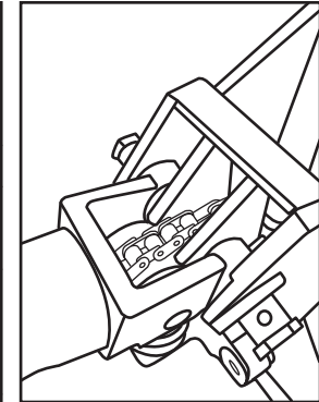
Pic. 3- The chain bolt should be in this position, slowly lift handle to upright position
