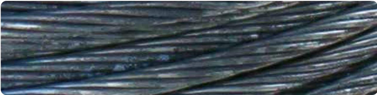
Figure 4: Oxidation on a conductor.
