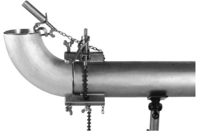
1. Mount the Clamp Champ onto the pipe end as shown in the earlier section. Position the jack screws so that the ball is even with the surface of the pipe.
