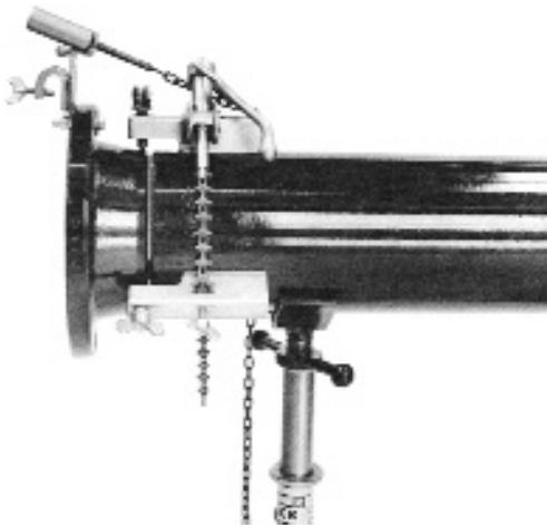
1. Mount the Clamp Champ onto the pipe end as shown in earlier section. Position the jack screws so that the ball is even with the surface of the pipe.
