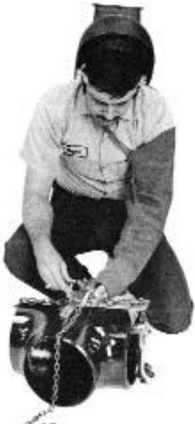
3. Rotate the adjustment knob on the leveling and supporting device so that approximately 2 inches (50mm) of threaded shaft is extended.
