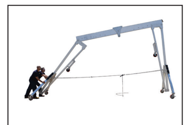
Ratchet 2nd A-Frame until it can be pushed into place.
