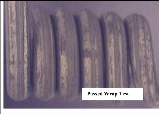
Figure IX: Beznal: Heat Treated at 250<sup>0</sup> C for a soak time of 6 Hours
