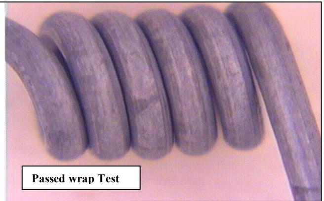
Figure XIV: Beznal: Heat Treated at 315<sup>0</sup> C for a soak time of 16 weeks.
