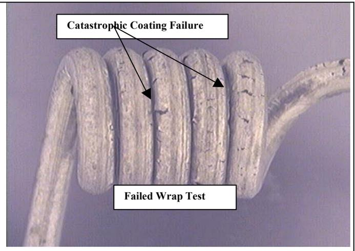
Figure VII: Galvanized: Heat Treated at 250<sup>0</sup> C for a soak time of 48 Hours (Two days)
