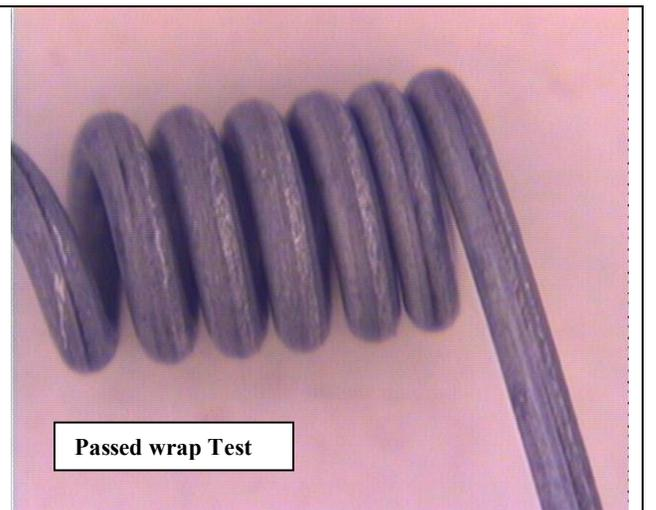
Figure XVI: Beznal: Heat Treated at 350<sup>0</sup> C
