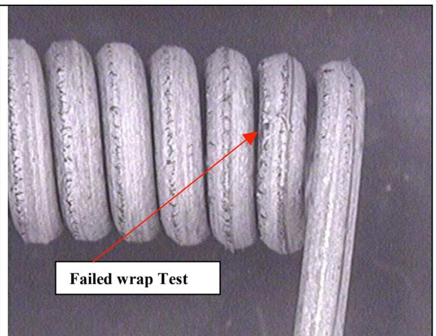
Figure IV: Galvanized: Heat Treated at 200<sup>0</sup> C for a soak time of Seven Weeks.
