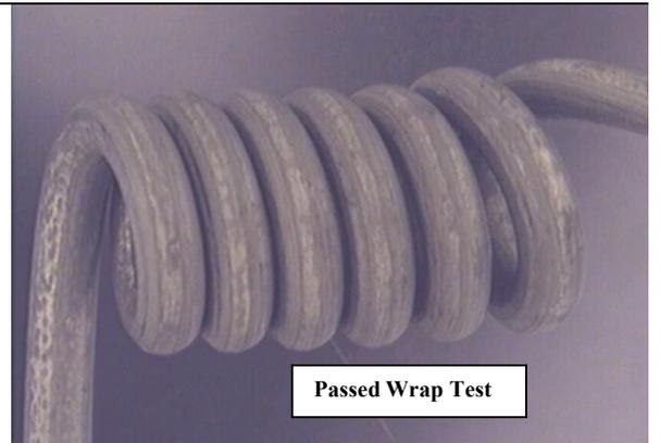
Figure XI: Galvanized: Heat Treated at 315<sup>0</sup> C for a soak time of 14 Hours
