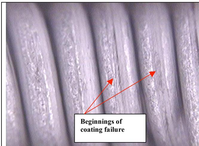
Figure III: Galvanized: Heat Treated at 200<sup>0</sup> C for a soak time of one five weeks.
