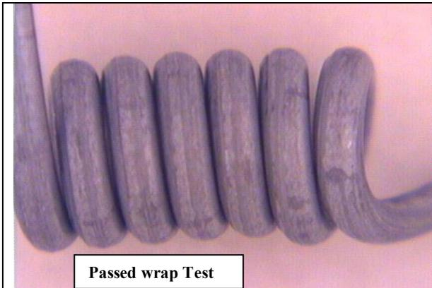
Figure XIII: Beznal: Heat Treated at 315<sup>0</sup> C for a soak time of 4 weeks.
