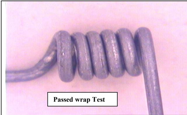
Figure V: Galvanized: Heat Treated at 215<sup>0</sup> C for a soak time of 14 hours.
