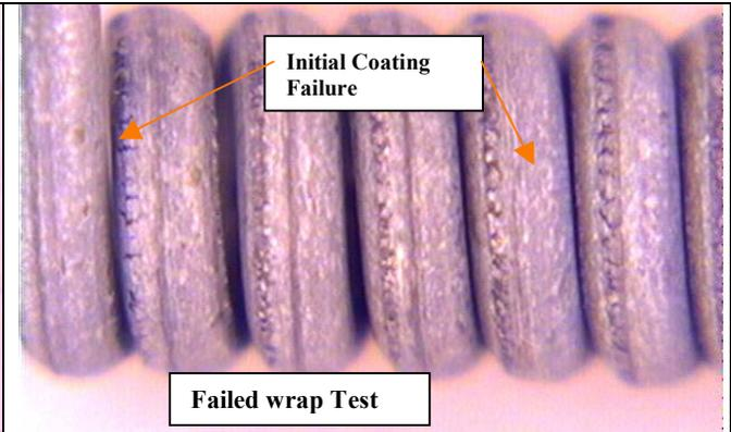
Figure VI: Galvanized: Heat Treated at 215<sup>0</sup> C for a soak time of 1 week.
