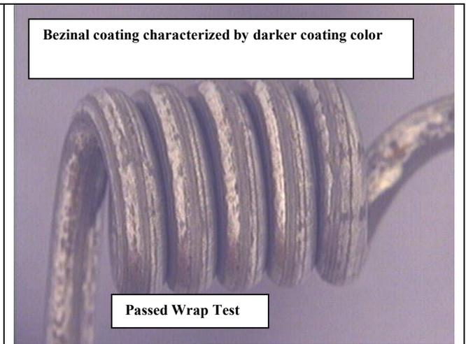
Figure I: Galvanized Coating: Pre Heat treated
