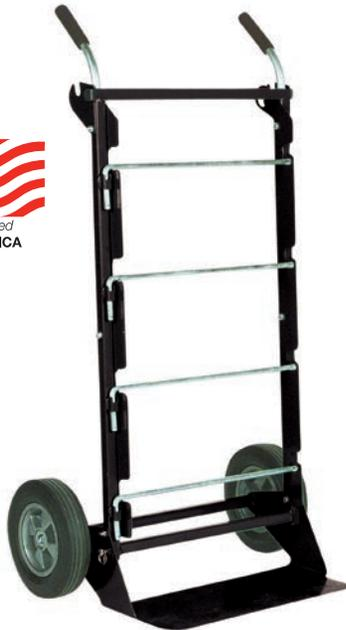
Transports spools on spindles and works as a dolly. Wire is dispensed while laying flat.
