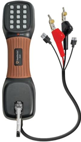
Rugged and cost-effective, the B600 Professional Telephone Test Set features Hi-Z monitoring, Pulse and Tone (DTMF), 10 number speed dial, and polarity indication in a rugged, double-molded housing.
