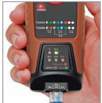
Illuminated LEDs and color wiring reference chart
