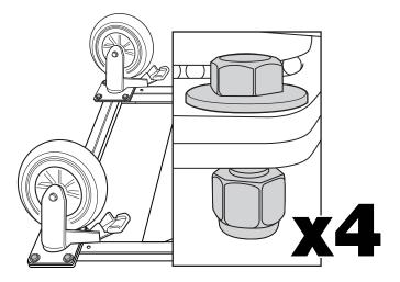
CAUTION: Do not over-tighten nylon lock nut, it will reduce holding ability.
