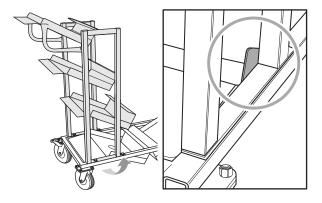
Fasten uprights to base using (1) 5/16 x 2" bolt, a 5/16" washer above and below frame, and (1) 5/16" nylon lock nut. Repeat step for 2nd upright
