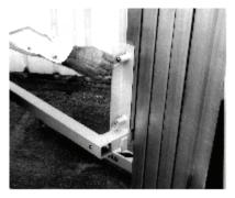
Disengage 4 spring-loaded pins. Rotate fork assembly 180 degrees. Engage 4 spring-loaded pins.
