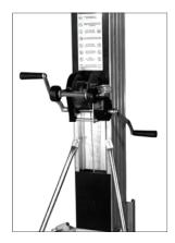
Use the winch to crank forks up or down into the desired position. Then crank winch handles up about 1/4 turn to set the safety brake.
