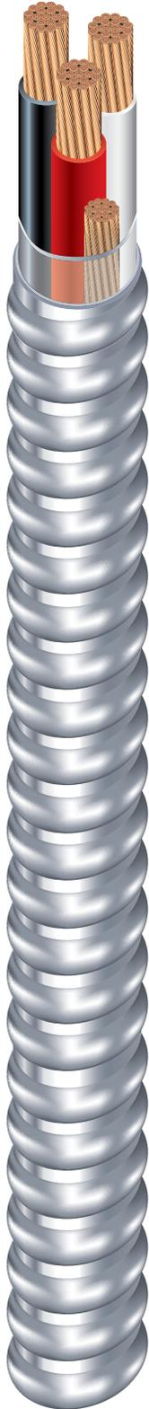
1 AWG through 750 kcmil Copper THHN/THWN-2 Insulated Singles. Copper Grounding Conductor. UL Listed. 600 Volts. Rated VW-1. Lightweight Aluminum Interlocked Armor.
