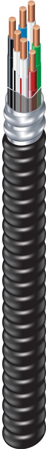
14 AWG through 8 AWG Copper THHN/THWN Insulated Singles. Dedicated Neutral Conductor for Each Phase Conductor. Green Copper THHN Insulated Grounding Conductor. UL Listed. 600 Volts. Rated VW-1. Lightweight Aluminum Interlocked Armor. Sunlight Resistant, Direct Burial Rated Overall PVC Jacket.
