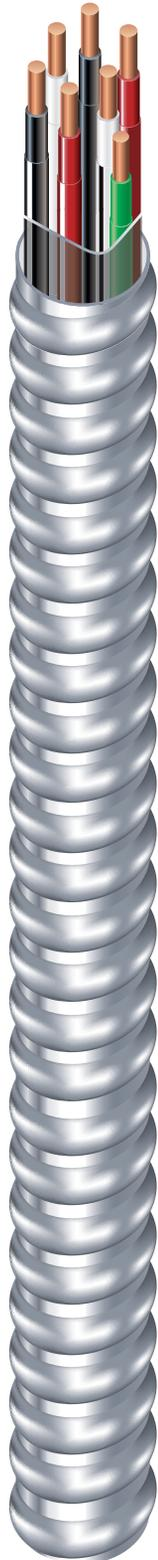
14 AWG through 10 AWG Copper THHN/THWN Insulated Singles. Multiple Circuits. Green Insulated Grounding Conductor. UL Listed. 600 Volts. Rated VW-1. Lightweight Aluminum Interlocked Armor.
