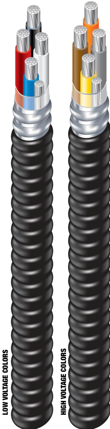
1/0 AWG through 900 kcmil AlumaFlex™ THHN/THWN-2 Insulated Singles with 8000 series Triple E™ Aluminum Alloy. Bare AlumaFlex™ Aluminum Alloy Grounding Conductor. UL Listed. 600 Volts. Lightweight Aluminum Interlocked Armor. Overall PVC Jacket.
