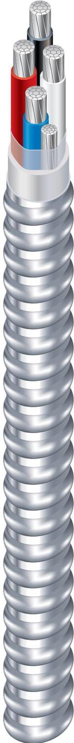
1/0 AWG through 900 kcmil AlumaFlex™ THHN/THWN-2 Insulated Singles with 8000 series Triple E™ Aluminum Alloy. Bare AlumaFlex™ Aluminum Alloy Grounding Conductor. UL Listed. 600 Volts. Binder Jacket for Continuous Conductor Support. Lightweight Aluminum Interlocked Armor.
