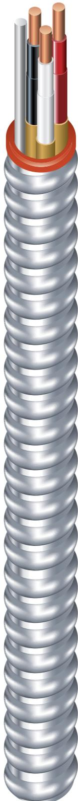
14 AWG through 2 AWG THHN/THWN Insulated Singles Wrapped in Moisture-Resistant, Flame-Retardant Paper. 16 AWG Aluminum Bond Wire. UL Listed. 600 Volts. Rated VW-1. Lightweight Aluminum Interlocked Armor.
