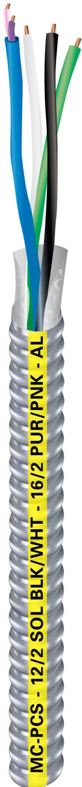
Copper Power & Control/Signal Conductors. Power: 12 AWG & 10 AWG Copper THHN/THWN Insulated Singles. Signal: 16 AWG Copper TFN Insulated Singles. Green Copper THHN Insulated Ground. UL Listed. 600 Volts. Rated VW-1. Lightweight Aluminum Interlocked Armor. Southwire® MC-PCS Duo™ Cable meets the NEC and UL listing requirements for combining power/lighting circuits and Class 2 or Class 3 signal or control circuits in the same cable.
