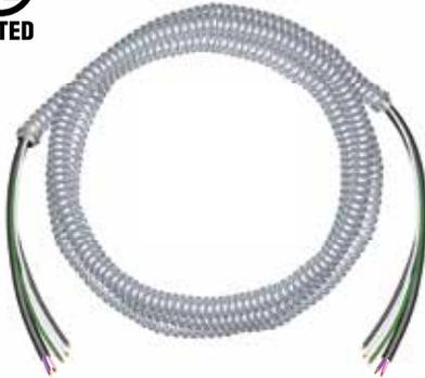
Interlocked Steel Armor with Factory Installed Conductors. Factory Installed Lock-nut or Snap-in Fittings. 600 Volts. Sizes 18 and 16 AWG Copper TFN or TFFN Conductors. Sizes 14 and 12 AWG Copper THHN/THWN Conductors. Green Insulated Copper Grounding Conductor.
