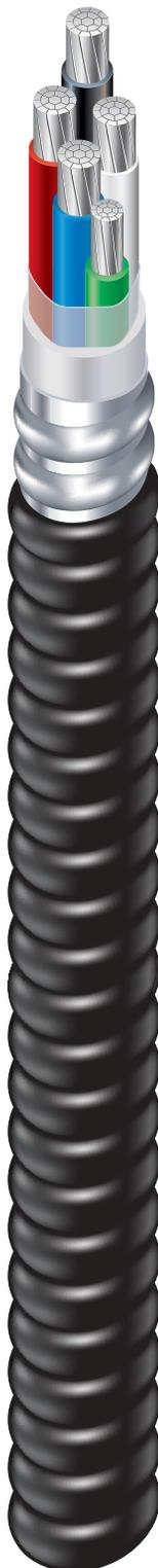
1/0 AWG through 900 kcmil AlumaFlex™ THHN/THWN-2 Insulated Singles with 8000 series Triple E™ Aluminum Alloy. Insulated green AlumaFlex™ Aluminum Alloy Grounding Conductor. UL Listed. 600 Volts. Binder Jacket for Continuous Conductor Support. Lightweight Aluminum Interlocked Armor. Overall PVC Jacket.
