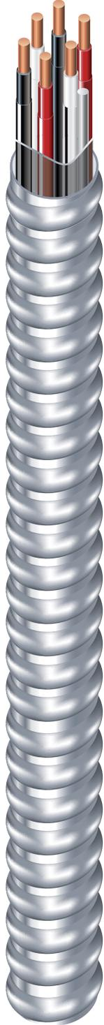
14 AWG through 10 AWG Copper THHN/THWN Insulated Singles. Full-Size Aluminum Equipment Grounding/Bonding Conductor. UL Listed. 600 Volts. Rated VW-1. Lightweight Aluminum Interlocked Armor is Part of Equipment Grounding/Bonding Path.
