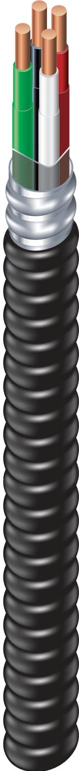
14 AWG through 2 AWG THHN/THWN Insulated Singles. Green Insulated Ground. UL Listed. 600 Volts. Rated VW-1. Lightweight Aluminum Interlocked Armor. Sunlight Resistant Overall PVC Jacket.
