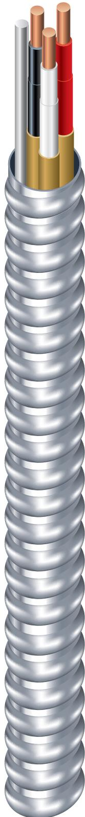
14 AWG through 2 AWG Copper Type ACTHH (THHN Singles). 16 AWG Aluminum Bond Wire. UL Listed. 600 Volts. Rated VW-1. Galvanized Steel Interlocking Armor.
