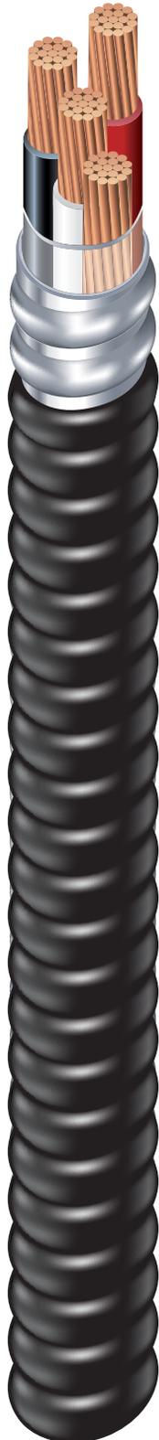
1 AWG through 750 kcmil Copper THHN/THWN-2 Insulated Power Feeder Conductors. Bare Copper Grounding Conductor. UL Listed. 600 Volts. Rated VW-1. Lightweight Aluminum Interlocked Armor with Overall PVC Jacket.
