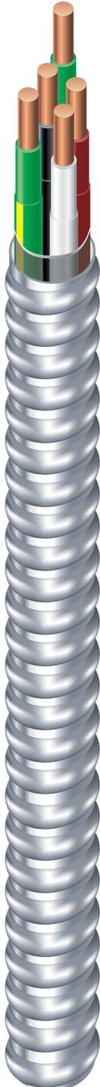
14 AWG through 8 AWG Copper THHN/THWN Insulated Conductors. Two Insulated Grounding Conductors. UL Listed. 600 Volts. Rated VW-1. Lightweight Aluminum Interlocked Armor.
