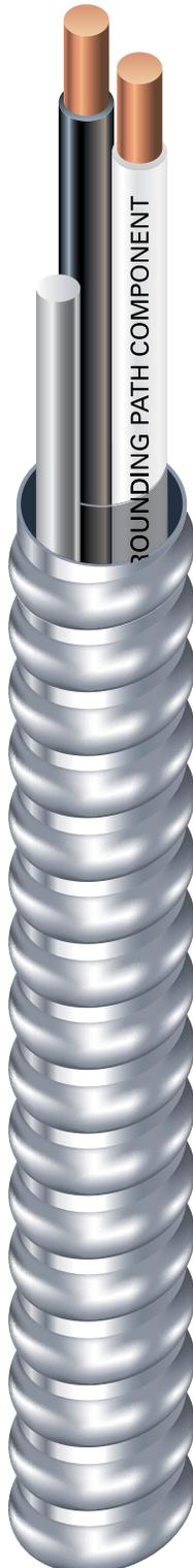
14 AWG through 8 AWG Copper THHN Insulated Conductors. Full-Sized Aluminum Equipment Grounding/Bonding Conductor. UL Listed. 600 Volt. Rated VW1. Lightweight Aluminum Interlocked Armor is Part of Equipment Bonding/Grounding Path.
