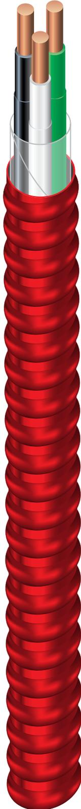
Sizes 14 & 12 AWG Type THHN/THWN Insulated Copper Singles. Sizes 18 & 16 AWG Type TFN Insulated Copper Singles. Green Insulated or Tinned Copper Grounding Conductor. UL Listed as Type MC and Type FPLP. 600 Volt Type MC and 300 Volt Type FPLP. Rated VW-1. Red Lightweight Aluminum Interlocked Armor.
