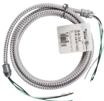
14 AWG through 10 AWG THHN/THWN Insulated Singles. Green Insulated Ground. UL Listed. 600 Volts. Rated VW-1. Lightweight Aluminum Interlocked Armor. Includes UL Listed Fittings and Prepared Cable Ends.
