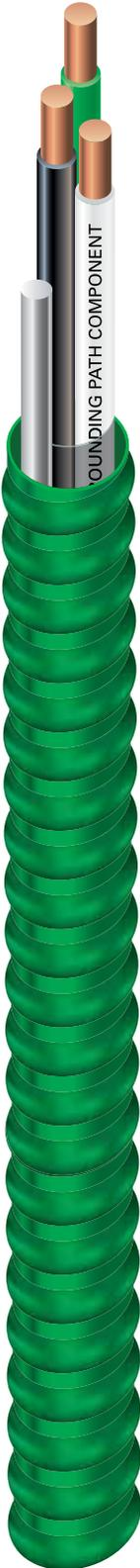
14 AWG through 8 AWG Copper THHN Insulated Conductors and Green Insulated Ground Conductor. Full-Size Aluminum Equipment Grounding/Bonding Conductor. UL Listed. 600 Volts. Rated VW-1. Galvanized Green Steel Interlocked Armor is Part of Equipment Bonding/Grounding Path.
