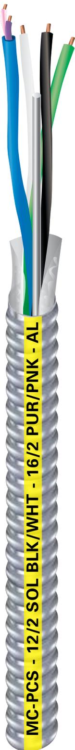
Copper Power & Control/Signal Conductors. Power: 12 AWG & 10 AWG Copper THHN/THWN Insulated Singles. Signal: 16 AWG Copper TFN Insulated Singles. Full-Sized Aluminum Equipment Grounding/Bonding Conductor. UL Listed. 600 Volts. Rated VW-1. Lightweight Aluminum Interlocked Armor is Part of Equipment Bonding/ Grounding Path. Southwire® MC-PCS Duo™ Cable meets the NEC and UL listing requirements for combining power/lighting circuits and Class 2 or Class 3 signal/control circuits in the same cable.
