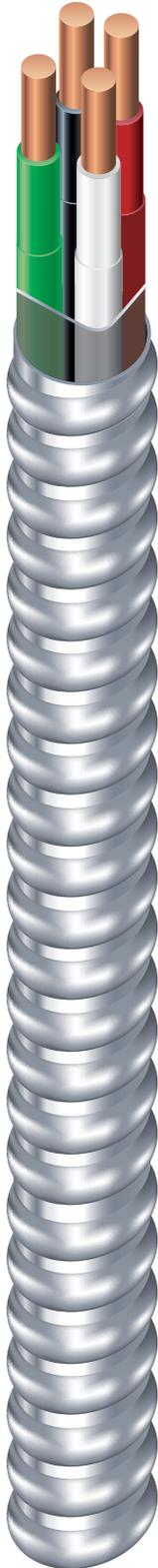
14 AWG through 6 AWG Copper THHN/THWN Insulated Singles. Green Copper THHN Insulated Grounding Conductor. UL Listed. 600 Volts. Rated VW-1. Lightweight Steel Interlocked Armor. Also available in Blue Steel Armor.
