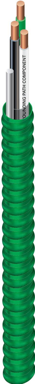
14 AWG through 8 AWG Copper THHN Insulated Conductors and Green Insulated Ground Conductor. Full-Sized Aluminum Equipment Grounding/Bonding Conductor. UL Listed. 600 Volts. Rated VW-1. Green Lightweight Aluminum Interlocked Armor is Part of Equipment Bonding/Grounding Path.
