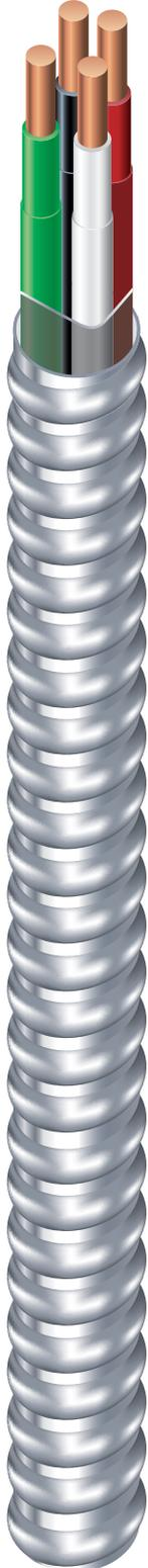
14 AWG through 2 AWG THHN/THWN Insulated Singles. Green Insulated Ground. UL Listed. 600 Volts. Rated VW-1. Lightweight Aluminum Interlocked Armor.
