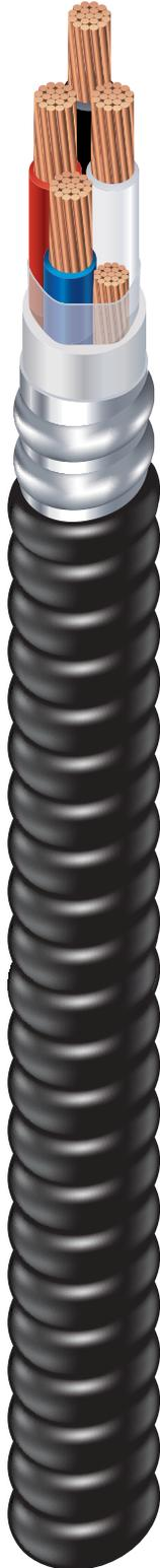
1/0 AWG through 750 kcmil Copper THHN/THWN-2 Insulated Singles. Bare Copper Grounding Conductor. UL Listed. 600 Volts. Binder Jacket for Continuous Conductor Support. Lightweight Aluminum Interlocked Armor with Overall PVC Jacket.
