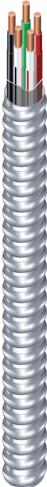
14 AWG through 8 AWG Copper THHN/THWN Insulated Singles. Dedicated Neutral Conductor for Each Phase Conductor. Green Copper THHN Insulated Grounding Conductor. UL Listed. 600 Volts. Rated VW-1. Lightweight Aluminum Interlocked Armor.
