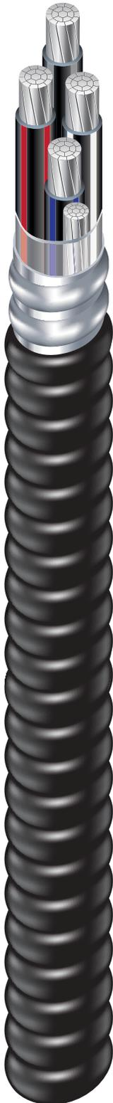
6 AWG through 900 kcmil XHHW-2 Insulated Singles with 8000 Series Triple E™ Aluminum Alloy. Bare AlumaFlex™ Aluminum Alloy Grounding Conductor. UL Listed. 600 Volts. Lightweight Aluminum Interlocked Armor with Overall PVC Jacket.
