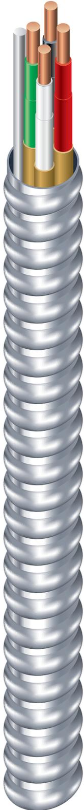
14 AWG through 10 AWG Copper Type ACTHH (THHN Singles). Green Copper Grounding Conductor. 16 AWG Aluminum Bond Wire. UL Listed. 600 Volts. Rated VW-1. Galvanized Steel Interlocked Armor. This product is a non-stock item and subject to minimum run quantities.
