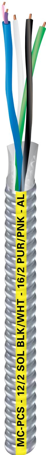
Copper Power & Control/Signal Conductors. Power: 12 AWG & 10 AWG Copper THHN/THWN Insulated Singles. Signal: 16 AWG Copper TFN Insulated Singles. Green Copper THHN Insulated Ground. UL Listed. 600 Volts. Rated VW-1. Lightweight Steel Interlocked Armor. Southwire® MC-PCS Duo™ Cable meets the NEC and UL listing requirements for combining power/lighting circuits and Class 2 or Class 3 signal or control circuits in the same cable.
