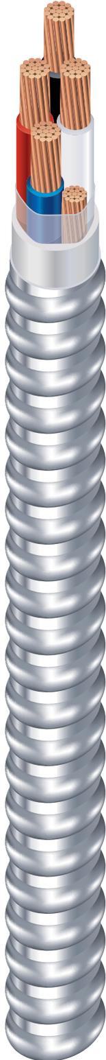
1/0 AWG through 750 kcmil Copper THHN/THWN-2 Insulated Singles. Bare Copper Grounding Conductor. UL Listed. 600 Volts. Binder Jacket for Continuous Conductor Support. Lightweight Aluminum Interlocked Armor.
