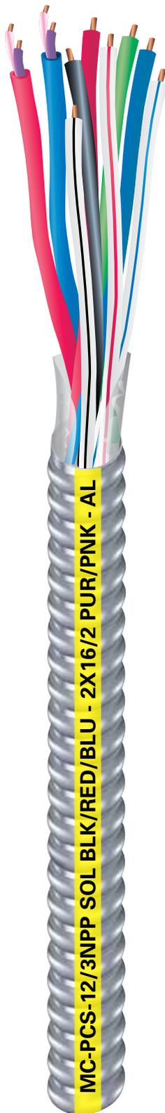
Copper Power & Control/Signal Conductors. Power: 12 AWG & 10 AWG Copper THHN/THWN Insulated Singles. Signal: 16 AWG Copper twisted jacketed pairs TFN insulated singles. Green Copper THHN Insulated Ground. UL Listed. 600 Volts. Rated VW-1. Lightweight Aluminum Interlocked Armor. Southwire® MC-PCS Duo™ Cable meets the NEC and UL listing requirements for combining power/lighting circuits and Class 2 or Class 3 signal or control circuits in the same cable.
