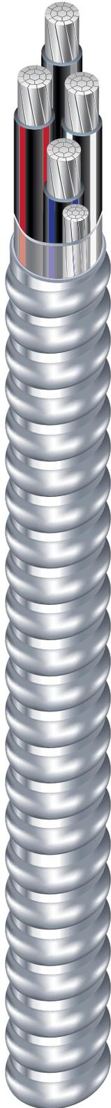
6 AWG through 900 kcmil AlumaFlex™ XHHW-2 Insulated Singles with 8000 series Triple E™ Aluminum Alloy. Bare AlumaFlex™ Aluminum Alloy Grounding Conductor. UL Listed. 600 Volts. Lightweight Aluminum Interlocked Armor.
