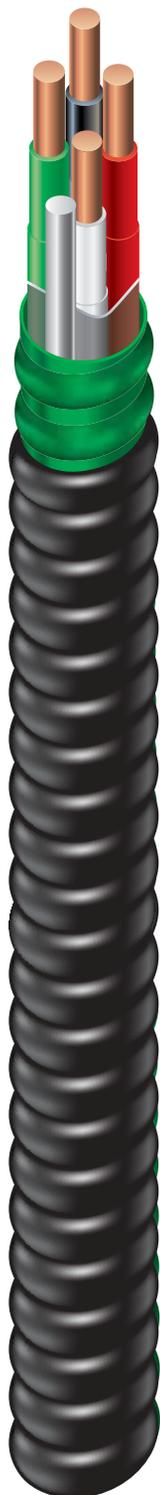
14 AWG through 8 AWG Copper THHN Insulated Conductors and Green Insulated Ground Conductor. Full-Sized Aluminum Equipment Grounding/Bonding Conductor. UL Listed. 600 Volts. Rated VW-1. Green Lightweight Aluminum Interlocked Armor is Part of Equipment Bonding/ Grounding Path. Sunlight Resistant, Direct Burial Overall PVC Jacket.
