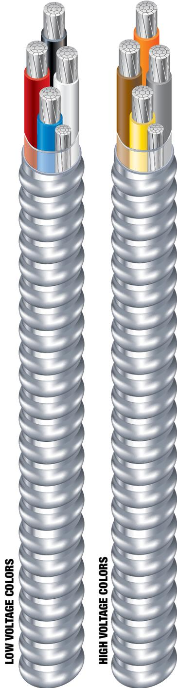
1/0 AWG through 900 kcmil AlumaFlex™ THHN/THWN-2 Insulated Singles with 8000 series Triple E™ Aluminum Alloy. Bare AlumaFlex™ Aluminum Alloy Grounding Conductor. UL Listed. 600 Volts. Lightweight Aluminum Interlocked Armor.
