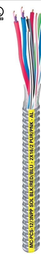
Copper Power & Control/Signal Conductors. Power: 12 AWG & 10 AWG Copper THHN/THWN Insulated Singles. Signal: 16 AWG Copper twisted jacketed pairs TFN insulated singles. Green Copper THHN Insulated Ground. UL Listed. 600 Volts. Rated VW-1. Lightweight Aluminum Interlocked Armor. Southwire<sup>®</sup> MC-PCS Duo™ Cable meets the NEC and UL listing requirements for combining power/lighting circuits and Class 2 or Class 3 signal or control circuits in the same cable.
