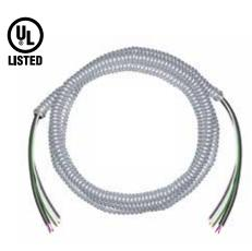
Interlocked Steel Armor with Factory Installed Conductors. Factory Installed Lock-nut or Snap-in Fittings. 600 Volts. Sizes 18 and 16 AWG Copper TFN or TFFN Conductors. Sizes 14 and 12 AWG Copper THHN/THWN Conductors. Green Insulated Copper Grounding Conductor.
