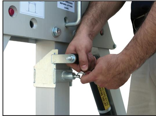
Release the plunger pin on the lifting handle and slide handle to desired position most convenient for lifting or lowering A-frame height. Release plunger pin and be certain it locks into place through pre-set holes before attempting to make height adjustment.
