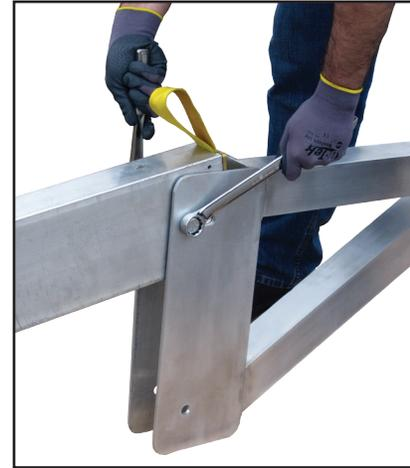
5. Place bolt through bolt hole on A-frame and cross beam with washers on either side of the bolt. Loosely tighten so A-frame can swivel when A-frame is erected.
