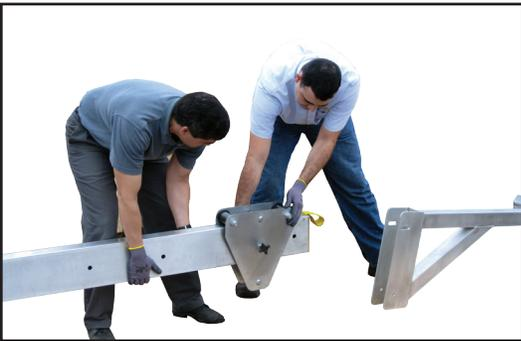
3. Place trolley at the opposite end of the cross beam. Center trolley on cross beam and tighten with set screw.
