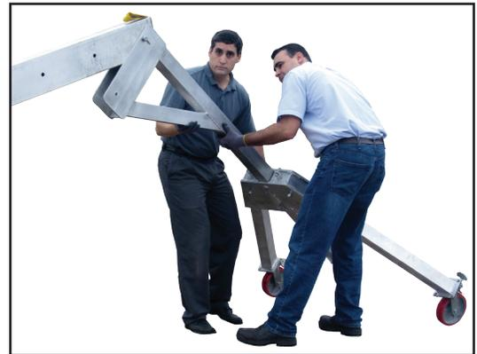
6. Erect one A-frame and line up inside bolt hole on the A-frame with corresponding bolt hole on the cross beam. Using a ladder, place bolt through bolt hole on A-frame and cross beam. Tighten both sets of bolts.
