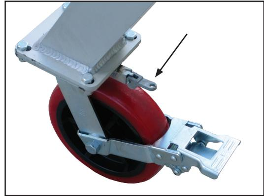
4. Casters can be locked at 90 degree angles to make transport easier. To lock caster at a 90 degree angle, flip the caster lock lever as indicated in above illustration.
