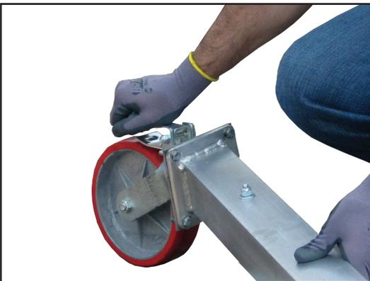
3. Lock all casters on both A-frames by pushing down on caster brake mechanism.
