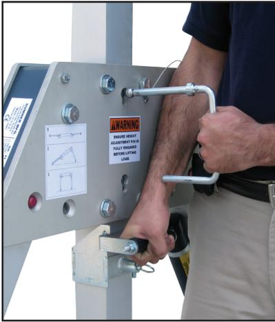
2. Once locking pin is removed, lift or lower A-frame to desired height. Replace locking pin.
