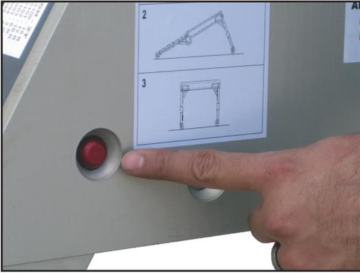
1. To extend one leg push the red leg locking button. The leg is now free to extend.
