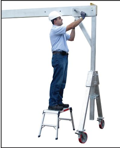
7. Erect second A-frame and line up inside bolt hole on the A-frame with corresponding bolt hole on the cross beam. Place bolt through bolt hole on A-frame and cross beam with washers on either side of the bolt. Fully tighten both sets of bolts.
