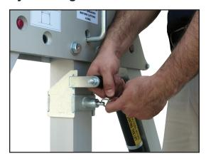
Release the plunger pin on the lifting handle and slide handle to desired position most convenient for lifting or lowering A-frame height. Release plunger pin and be certain it locks into place through pre-set holes before attempting to make height adjustment.
