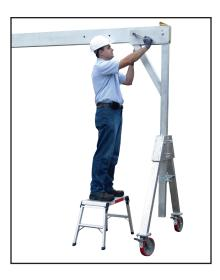
7. Erect second A-frame and line up inside bolt hole on the A-frame with corresponding bolt hole on the cross beam. Place bolt through bolt hole on Aframe and cross beam with washers on either side of the bolt. Fully tighten both sets of bolts.
