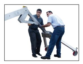
Erect one A-frame and line up inside bolt hole on the A-frame with corresponding bolt hole on the cross beam. Using a ladder, place bolt through bolt hole on A-frame and cross beam. Tighten both sets of bolts.
