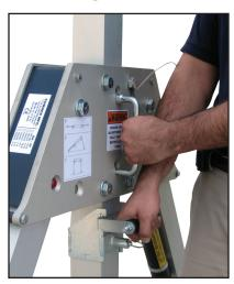
1. With one hand lift on lifting handle. Remove locking pin with other hand.
