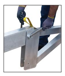
Place bolt through bolt hole on A-frame and cross beam with washers on either side of the bolt. Loosely tighten so A-frame can swivel when Aframe is erected.
