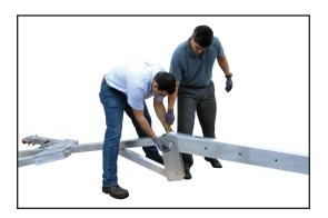
Lift one side of cross beam onto A-frame and line up outside bolt hole on A-frame with desired bolt hole on cross beam. Place bolt through bolt hole on A-frame and cross beam with washers on either side of the bolt. Loosely tighten so A-frame can swivel when A-frame is erected.
