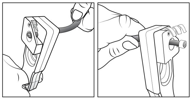
5. Once desired length of strip length is obtained, slide a finger of opposite hand against back side of stripper to stop advancement of the stripper. Continue to rotate until jacket material is rounded off.
