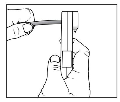
2. For sizes #6-#4awg, Insert cable until it is flush with the front of the wire support body. For sizes #3awg-1/0, insert cable until the edge of the jacket is in the center of the stripping blade.
