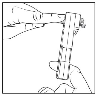
6. Pull down on the spring loaded finger trigger and slide stripper off of the cable.
