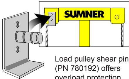
Load pulley shear pin (PN 780192) offers overload protection. Each Roust-A-Bout comes with a spare for quick, in-field resetting.
