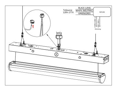
5. Insert the conduit cable and fully secure.
