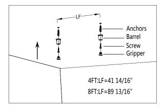
2. Then, tighten gripper back to the barrel and adjust to desired length of cable. Clip-on to the keyholes of the fixture.
