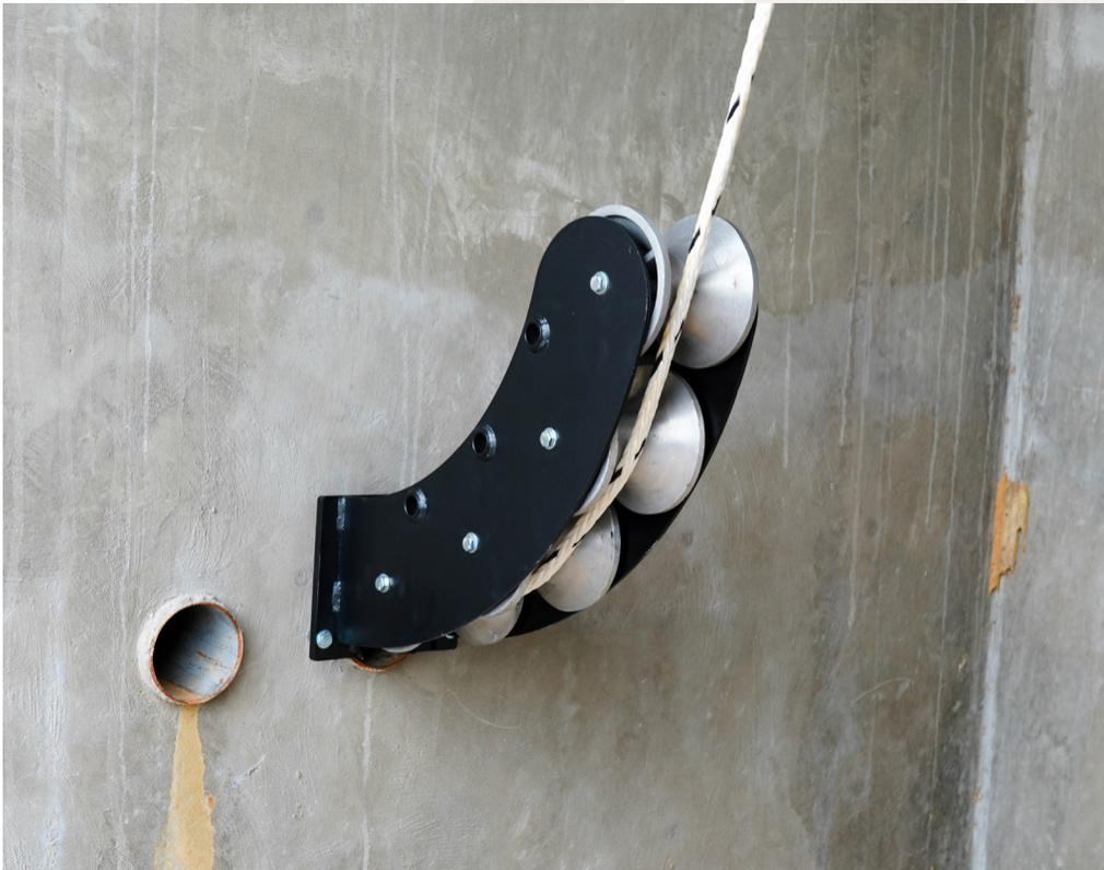
**ASSIST IN GUIDING CABLE INTO DUCTS OR CONDUIT**
