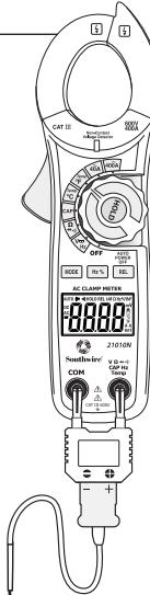
**⚠ WARNING:** To avoid electric shock, remove the temperature probe before changing to another measurement function.
