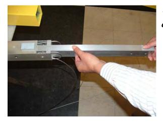
*12. Remove top mast tube from center mast.*
