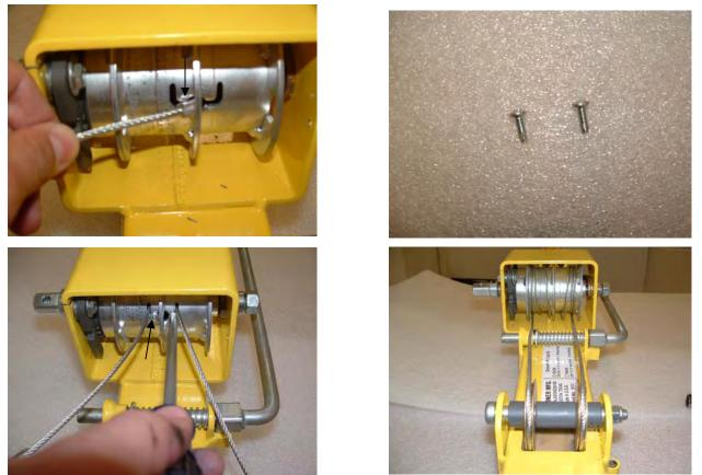
*30. Insert cables in drum and secure with (776042) screws as shown. \*Once cables are secure weave the excess cable on the drum.*
