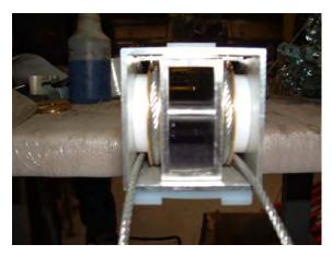
21. Insert top mast assembly into center mast tube by pulling both cables at the same time and stop when the end of the top mast passes the second hole of the center mast tube.
