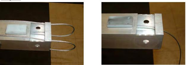
10. Pull cable from the loop position to a strait position through the bottom of the center mast for easy removal of top mast assembly.
