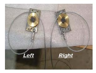
*13. Remove (784399) center mast pulley weldments from center mast and replace damaged cable as shown.*
