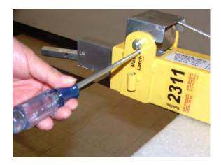
3. Remove (776042) screws and (784408) pulley guard.
