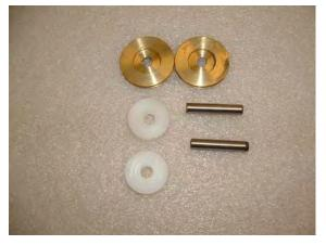
*19. Locate (784412) top mast wear discs, (784391) 2 " pulleys and (774041) dowel pins.*
