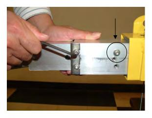
28. Locate (771044) screws, (773550) 1/4 lock washer, (784403) top covers and assemble them in both sides as shown. \*The lock washer goes on the single screw circled. This screw must be in the correct position for proper operation.
