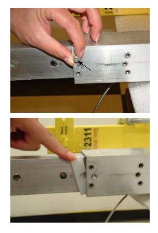
25. Insert (774452) wear pads into slots on both sides as shown.
