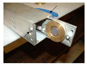
*16. Locate (771044) screws and secure the (784399) center mast pulley weldments brackets on both sides as shown.*
