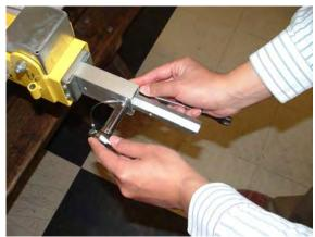
*33.* Assemble mast hold down assembly into the top mast and secure with (771055) screw and (772502) jam nut.
