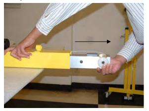
8. Remove center mast assembly from the bottom of the outer mast.
