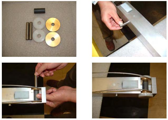
23. Locate (784404) center mast wear discs, (784390) 2-1/4" pulleys, (774043) dowel pins and (784447) 1-5/8" pulley spacer. Assemble components as shown.
