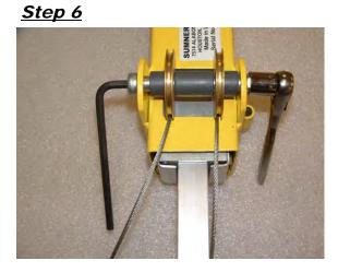
6. Remove top outer mast components as shown.
