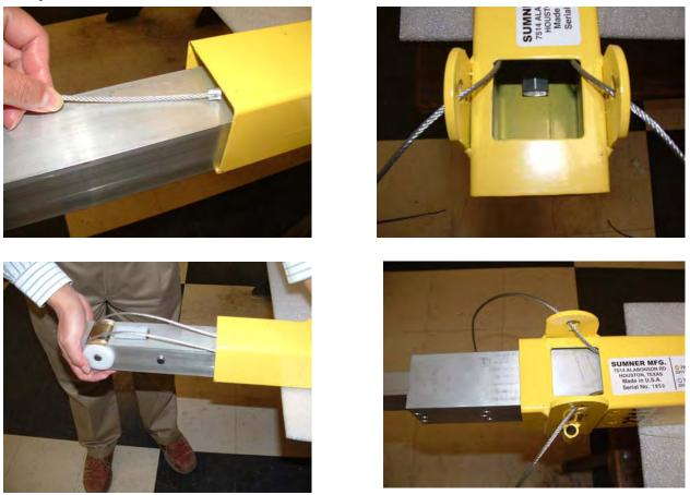
27. Insert both cables through the outer mast weldment as shown. \*Feed the cable all the way to the top of the outer mast.
