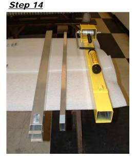
14. Lay down all mast sections on a solid level work surface. Make sure all components required to assemble the 2300 lift are at hand.
