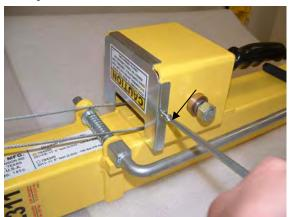
4. Remove (776042) screws and (774428) winch cover.
