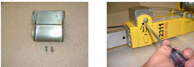
*31. Locate (784408) pulley guard, (776042) screws and assemble as shown.*
