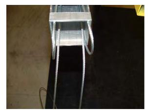
17. Straight cable on both sides as shown. Make sure cable is not tangle up inside the mast section.
