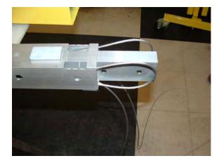
11. Pull top mast assembly slightly out the bottom mast of the center mast as shown and remove all components.
