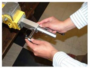
2. Remove mast hold down assembly, (771055) screw and (772502) jam nut.
