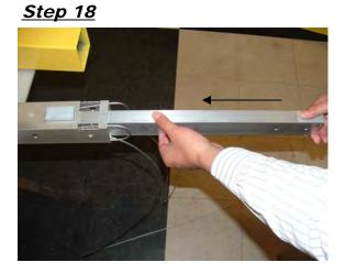
18. Insert top mast tube into center mast tube as shown.
