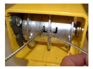
5. Remove (776042) screws from winch drum and remove cable as shown.
