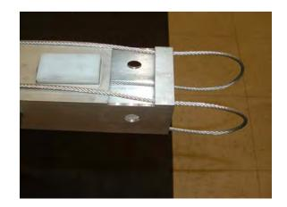
22. Insert and loop cable through the center mast slot as shown.
