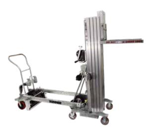
The Sumner\* Series 2500 lift is an inovative counter balance lift that features a compact design.
