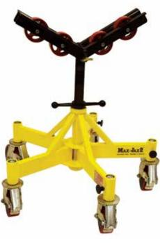
The Sumner\* MAX JAX\* 2 upgraded fabrication stands are the ideal high and low stand for fit-up, rotating and welding.
