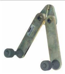
The Sumner\* Adjust-A-Flange<sup>™</sup> when used with the Adjust-A-Fit<sup>™</sup> is an alignment tool for fittings that uses gravity to make lining up fittings a trouble-free one man operation
