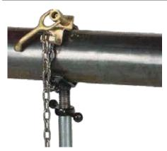
The Sumner\* Hold Down Device is ideal for securing material on vee head jacks for transportation and fit-ups.
