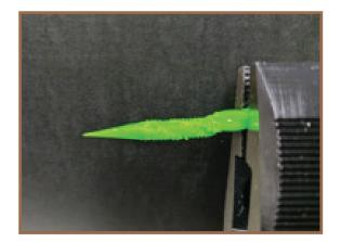
**STEP 4**: Using gloves, apply glue to the inside of replacement leader and quickly screw the replacement leader onto the fish tape material until the leader cannot be threaded on any further (This applies for the flexible metal leaders and the non-conductive leaders). After the leader is securely fastened, add one drop of glue to the base of the connection. Let leader set for 15 mins prior to usage.
