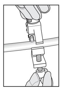
5. Engage V shape cable clamp by turning cable sizing thumb screw clockwise until cable is secured.
