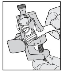
8B. **For Mid-Span** place a gloved hand against unibody frame while continuing to turn stripper clockwise.
