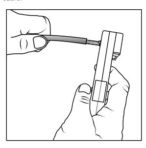
7. Depending on wire size there may be a little jacket material left on the very end of the cable. Slide this off with your fingers and strip is complete.
