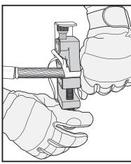
Release V shape cable clamp by turning counter clockwise to remove stripper.
