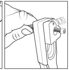
Once desired length of strip length is obtained, slide a finger of opposite hand against back side of stripper to stop advancement of the stripper. Continue to rotate until jacket material is rounded off.
