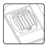
3. Complete installation with mounting bracket and replace lamp lens
