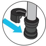
*TO REMOVE THE SIMPush<sup>™</sup> FITTING, SIMPLY SLIDE THE REMOVAL TOOL ONTO THE COLLAR AND PULL*
