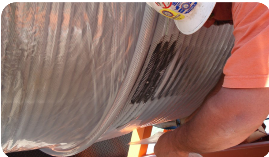
Figure 4: Oxidation on a conductor.
