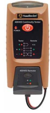
The Southwire 40040S provides a simple way of checking continuity on wire and cables. The bright LEDs and loud pulsating beeper provide a positive indication of continuity and polarity. A detachable remote indicator is included for tracing multiple cable runs.
