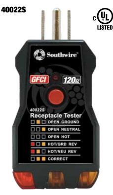
GFCI receptacle tester quickly identifies the most common wiring faults associated with 3-wire 120V outlets. Just plug it into the outlet and the indicator lights quickly tell you if the outlet is wired correctly. Press the red button to verify that a GFCI circuit is functioning properly.
