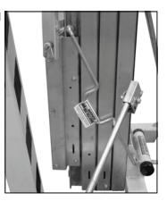
The winch handles have been placed in the stored position.
