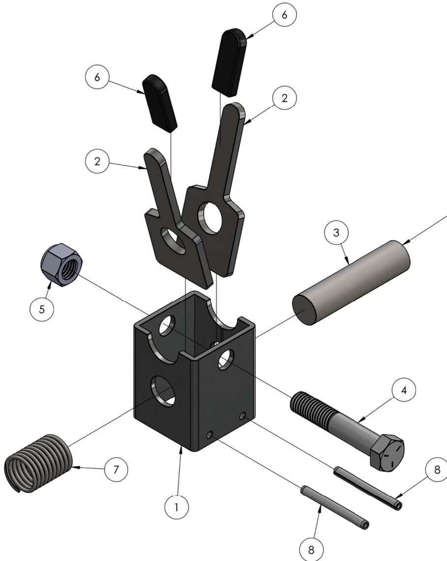
OUTRIGGER SUPPORT TUBE STUB LOCKS ASSEMBLY IS INSTALLED TO SUPPORT THE ASSEMBLY DURING SHIPMENT AND IS TO BE DISCARDED BEFORE INSTALLATION.
