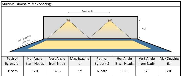
Application Notes: Calculations based on initial conditions, a 100-foot long corridor, 8-foot wide and 9-foot high, with 80/50/20 reflectances. Measurements at floor height. Illumination requirements were: average illuminance of no less than 1 fc, minimum illuminance of no less than 0.1 fc, and max/min ratio of no greater than 40:1.
