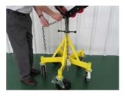
2. Back off adjustment screw in order to have maximum thread travel
