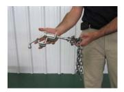
3. Insert chain into slot on Hold Down Housing and tighten adjustment screw.
