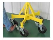
C. Make sure all casters are in the same direction. If not move each end of the Max Jax load in a circle to align casters
