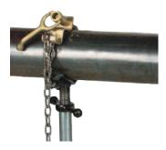
Insert chain end of hold down device through containment loop and tighten set screw to half the length of chain
