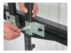
To clamp wide loads, plunger pin on the clamp forks should be positioned out towards the end of the head.
