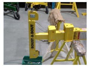
6. Insert top mast into center mast leaving 8 to12 inches of the top mast extended. Take care not to push in the center mast.
