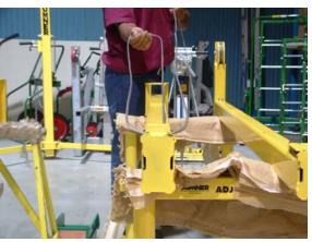
4. Take the end of the mast elevation line and insert the line around the pulley.
