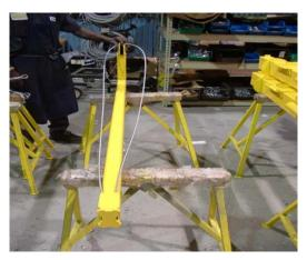
2. Take both ends of the equalizing line and place them underneath the top mast keeper plate as shown. Then secure both ends with a piece of wire . Place the looped end of the cable over the t-head for ease of assembly.
