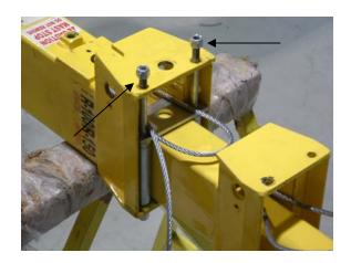
9. Insert (780022) bottom mast roller shafts and (780021) bottom mast rollers from the bottom. Secure the shaft with (772355) nut. \*Note: Hand tighten nut.
