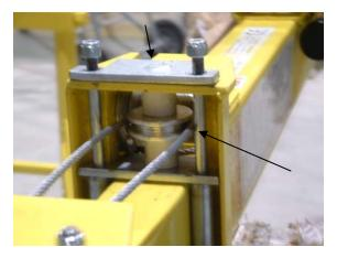
\*Note: You must remove nuts on roller shafts to insert shaft stay weldment. Take care not to allow roller shafts to drop out.
