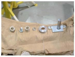
17. Retrieve (780295) shaft stay weldment, (780023) separator, 780293 separator, (780297) 2 inch pulley, (771125) bolt and (773590) lock washer. Place pulley into loop at end of equalizing line. Insert one separator on top and bottom of pulley as shown. Align with move in bottom mast. Insert shaft and secure with bolt and lock washer.
