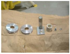
16. Retrieve (780299) 2-1/2 inch equalizing pulleys, (780343) separator, (780036) center mast shaft stay, (771020) bolt and (773550) lock washer . Place one pulley into each loop created in step 15. Align pulleys with holes in center mast. Insert shaft through pulleys making sure to place separator between pulleys. Secure with bolt and lock washer.
