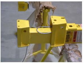
5. Insert center mast into the bottom mast leaving 8 to 12 inches of the center mast extended. Make sure the "loop" of the elevation line is visible.
