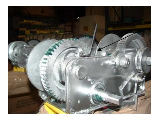
20. Insert mast elevation line into hoist drum. Secure the line with the set screw and wind the cable.
