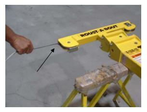
21. Feed the load line through the tee head assembly. From front to back.
