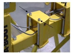
11. Assemble (780334) center mast roller shaft, (780349) center mast roller and nut as shown. Secure the shaft with (772355) nut. \*Note: Rollers are placed so cable is between them.
