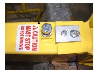
18. Take (771125) stop bolt, (773590) lock washer and assemble in the bottom mast.
