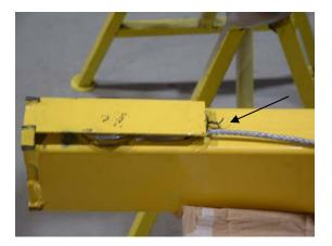
3. Take the mast elevation line button and place it underneath the center mast keeper plate as shown. Then secure the line with a piece of wire as shown.
