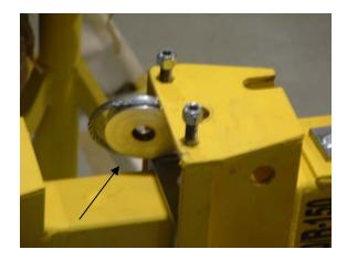
14. Retrieve (780299) 2-1/2 inch equalizing pulley, (780292) separator, (780198) bottom mast shaft, (773550) lock washer and (771020) bolt. Loop elevating line around pulley (bottom to top). Extend elevating line towards the bottom of the Roust-A-Bout. Align the center of the pulley and the hole in the side of the bottom mast. Insert shaft and separator and secure with bolt and lock washer.
