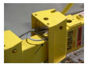
8. Insert (780090) bottom mast shaft plate underneath the cable as shown.
