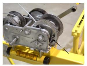
22. Repeat the same instructions as shown in step 1. Again, make sure the cable is wound over the top of the drum.
