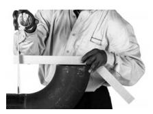
The **Mul-T-Square** consists of two 45° blades which slide effortlessly in an industrial grade plastic holder. Each blade is made of durable aircraft grade aluminum, trued for precise alignment. The 10" and 14" blade arms allow measurement of tight fitups or can be expanded for 30" squaring of 90° fittings. In some instances, the 45° blades are handy by themselves for simple alignment
