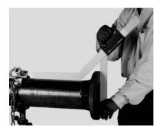
The sides of the **Mul-T-Square** handle are a compbination of 45° and 90° angles for quick alignment or marking. the handle opening can accommodate a gloved hand and the blade locking know is convenient to the operator's thumb. Blades can be loosened or secured by a single rotation of the licking knob.
