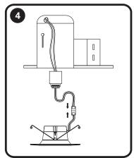
**Step 6:** Carefully route wires into fixture and push recessed kit up until flush with ceiling surface.
