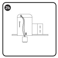
**Step 3:** Disconnect the included Edison base adaptor from the LED downlight and screw Edison base adaptor into socket in recessed housing.
