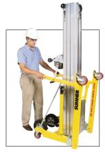
One piece slide-lock mechanism releases with plunger pins to fold legs. Leg rollers allow lift to be wheeled around with legs in stored position.
