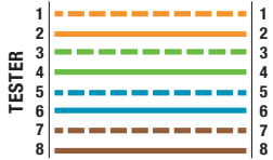
T568B Data Cable With a Shorted and Open Pair
