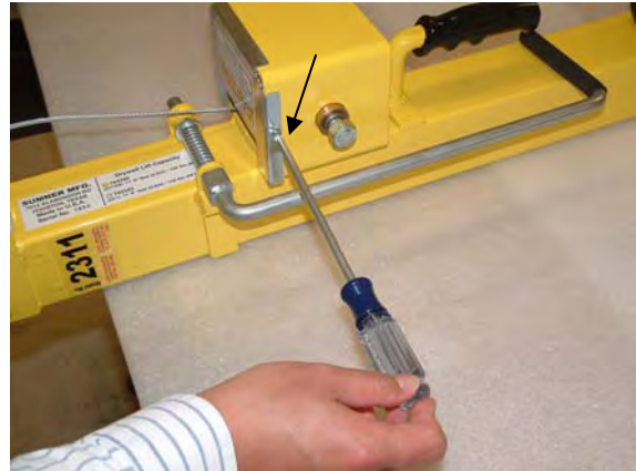
Assemble (784428) winch cover and secure with (776042) screws.
