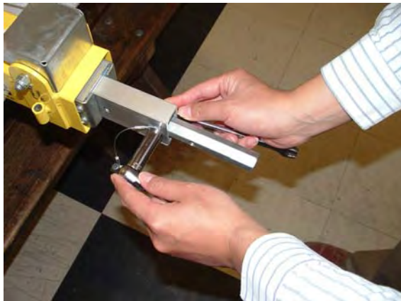
Assemble mast hold down assembly into the top mast and secure with (771055) screw and (772502) jam nut.
