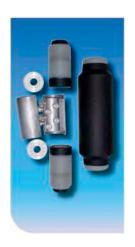
This premolded joint in three-piece design with compact dimensions is made of silicone rubber. Main components of the standard joint are conductor connection, cable adapters, main joint sleeve, and outer protective covering.
