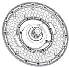
1. Remove sensor cap by rotating counterclockwise and lifting outward.
