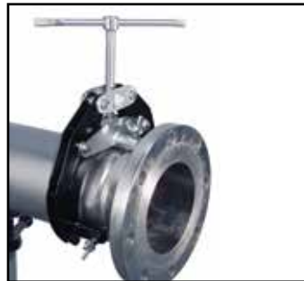
Pipe to flange
